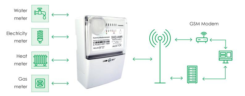
Meter Interface: RS232, RS485, CL (current loop), optional WMBus Meter Interface speed: 300 to 38400 baud, fix or MODE C **Configuration:** Locally or remotely **WAN Interface:** 4G, NB-IoT, LTE CatM, LTE450 Un 100-230 V AC, Fn 50 Hz or optional battery Power supply: Power consumption: max 1.5 W **GSM** antenna port: Nominal impedance: 50 Ohm; SMA/FME connector Operating temperature: -20°C to +85°C (>55°C derating) **Humidity:** 0-95%, non-condensing Housing: DIN standard; IP2x, UL94-V0
